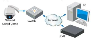
Figure 3-1 Wiring Over a LAN
